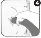
Place the vacuum hose over the valve to vacuum out the air.
